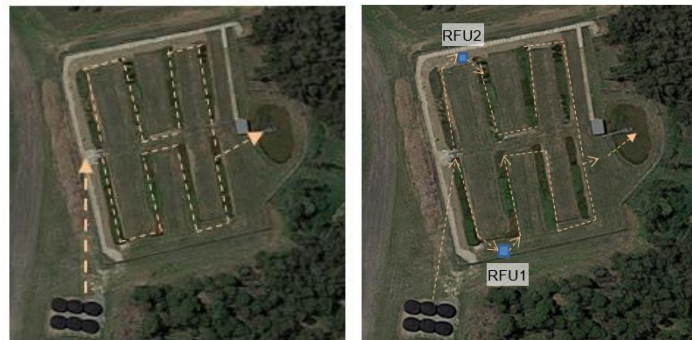
Figure 1. Existing vegetated swales for leachate treatment (left) and proposed RFUs (non-vegetated treatment to existing system) (right)
